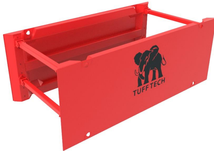
Image: TT-77 : M-1.5 Shoring, STAND-ALONE configuration, 4.0 meter long, 2.0 meter face-face
